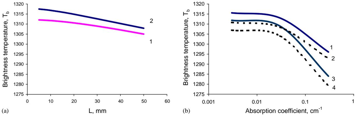
Fig. 3. Changing of brightness temperature with sample length for  $\alpha_1 = 0.02 \text{ cm}^{-1}$ : (a) 1—2D model [22]; 2—1D model [5]; with absorption coefficient  $\alpha_1$  for sample length equal to 4 cm (b) 1,3— $T_i = 1323 \text{ K}$ ; 2,4— $T_i = 1318 \text{ K}$ ; 1,2—2D model [22]; 3,4—1D model [5].
