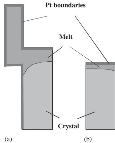
Fig. 2. Geometry of calculation domain in crystal growth via crucible pulling with a crystal downwards (a) and via the cooling method of the AHP heater (b).
