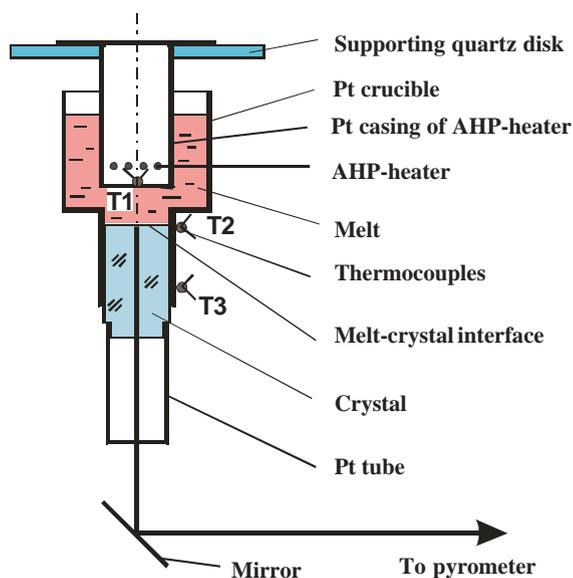
Fig. 1. Schematic of AHP crystallizer for measurements of interfacial undercooling.
